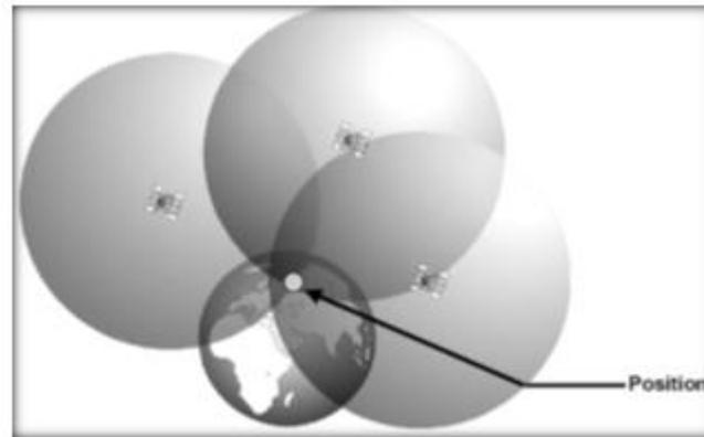
Figure 2.3: The intersection Point indicates the location of the GPS receiver[11]
