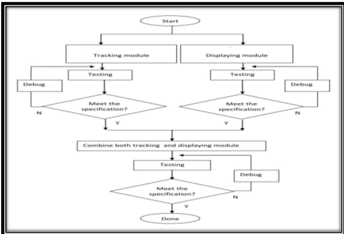
Figure 4.1 Testing flow of people tracing system
